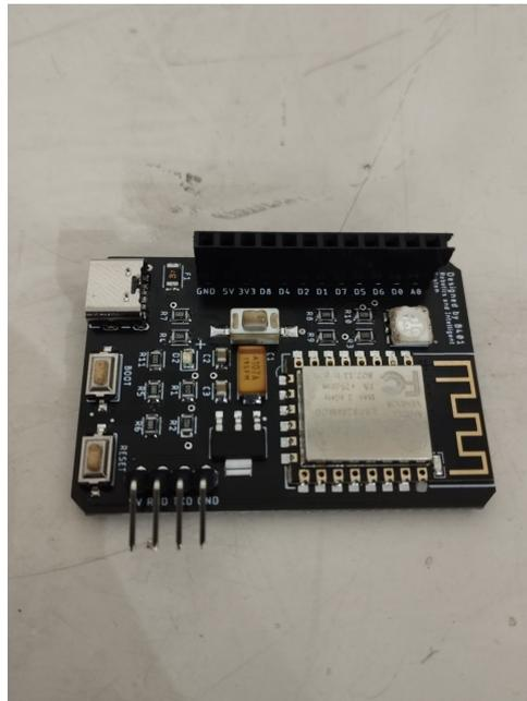
Gambar 4.8: Keadaan Board Setelah Solder Header Pin
